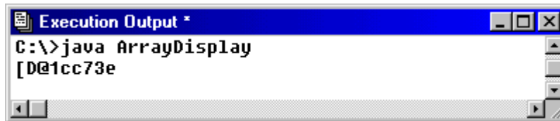
Figure 2.16: Result of using System.out.println on an array
